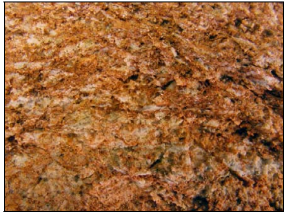
Fig. 4.5-8: Left - Sand/sandstone cemented by Fe-oxides, OP-2 borehole 6.3-6.4 m; Right – weathering residua (aluvium) of crystalline rock, probably migmatite, OP-2 borehole, 7.6-7.8 m. Areas shown on both photographs are 2.2 x 3 cm.
