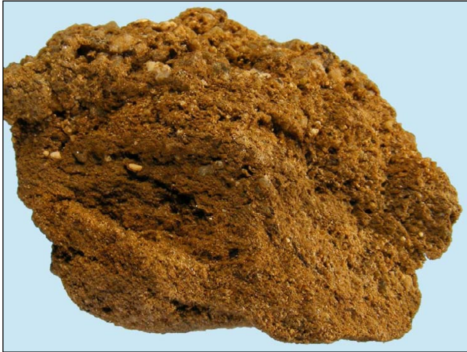
Fig. 4.5-13: Characteristic colluvial/alluvial sands from borehole OP-5 (depth 3.4 m) Size 5×4 cm.
