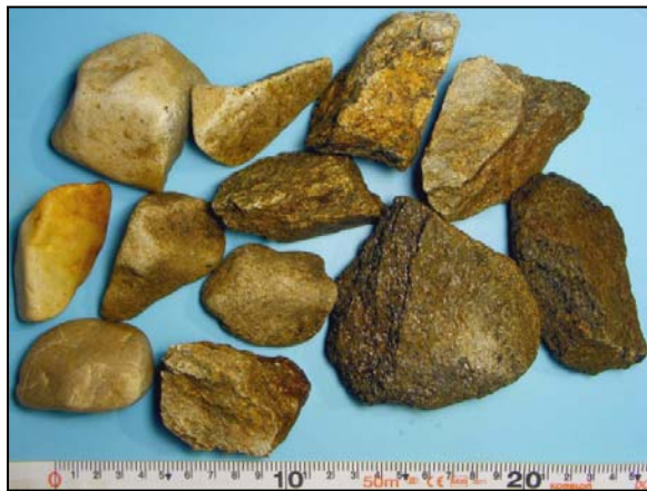
Fig. 4.5-13: Characteristic colluvial/alluvial sands from borehole OP-5 (depth 3.4 m) Size 5×4 cm.
