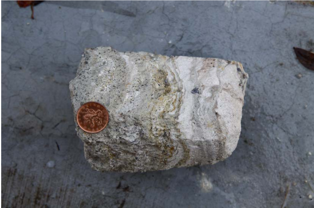
Fig. 4.4.1-5. Photograph of part of the core from HL-6 borehole, cut along two perpendicular planes. Kaolinic sands/sandstones, probably belonging to the Klikov Fm., display sub-horizontal bedding. The bending of the strata is a result of core deformation during drilling.
