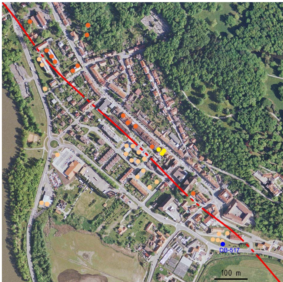
Fig. 4.3.3-1: Situation in the Hluboká-town section showing the boreholes used for mapping of the fault, colour-coded according to the stratigraphy of the Quaternary subcrop: cream yellow – sediments of the Klikov or Mydlovary Fm. (non-differentiated), brick red – crystalline, yellow – probably sandstones of the Zliv Fm. Borehole HRC-1 (DB-517) referred to in text shown as blue dot. Approximate inferred position of the Hluboká Fault shown by red line.
