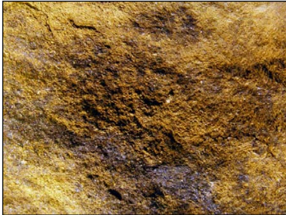
Fig. 4.5-8: Left - Sand/sandstone cemented by Fe-oxides, OP-2 borehole 6.3-6.4 m; Right – weathering residua (aluvium) of crystalline rock, probably migmatite, OP-2 borehole, 7.6-7.8 m. Areas shown on both photographs are 2.2 x 3 cm.
