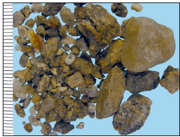
Fig. 4.5-13: Characteristic colluvial/alluvial sands from borehole OP-5 (depth 3.4 m) Size 5×4 cm.
